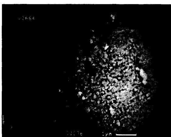
Fig. 5. Scanning electron micrographs of a LiChrosphere surface after polymer coating using the 40°C process (a); (b) after prolonged use in a column.
