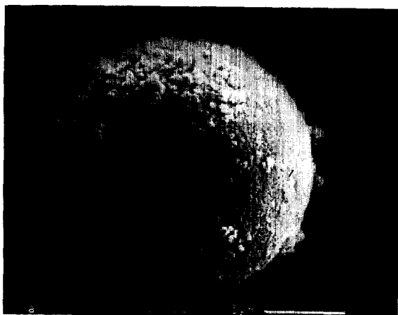
Fig. 3. Scanning electron micrograph of LiChrosphere 1000 before derivatization. Particle washed with 5% nitric acid and oven-dried at 140°C.
